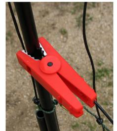
10. To open the fence to retrieve goods, unclip the red lead wire and clip it to the plastic post #1 again taking away the current. Remember not to touch any of the metal on the clip as it will shock you.
