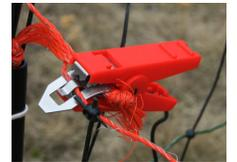
9. Unclip the red lead wire from the plastic post and clip it to the metal tab that is attached to the orange wires next to post #1. The fence is now live.
