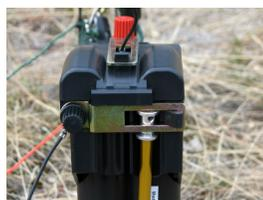
3. Attach the black (ground) lead wire to the energizer by placing the connector at the end of the wire on the ground terminal by removing
